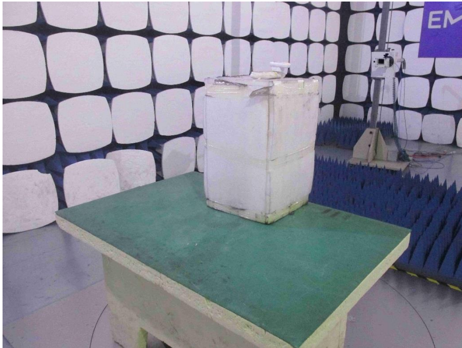
Photograph 4: Set-up for Conducted Emission on AC Mains
