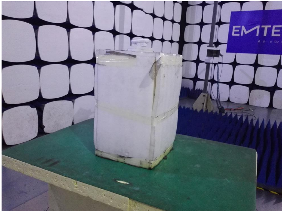
Photograph 2: Set-up for Radiated Spurious Emission, 1GHz - 18GHz
