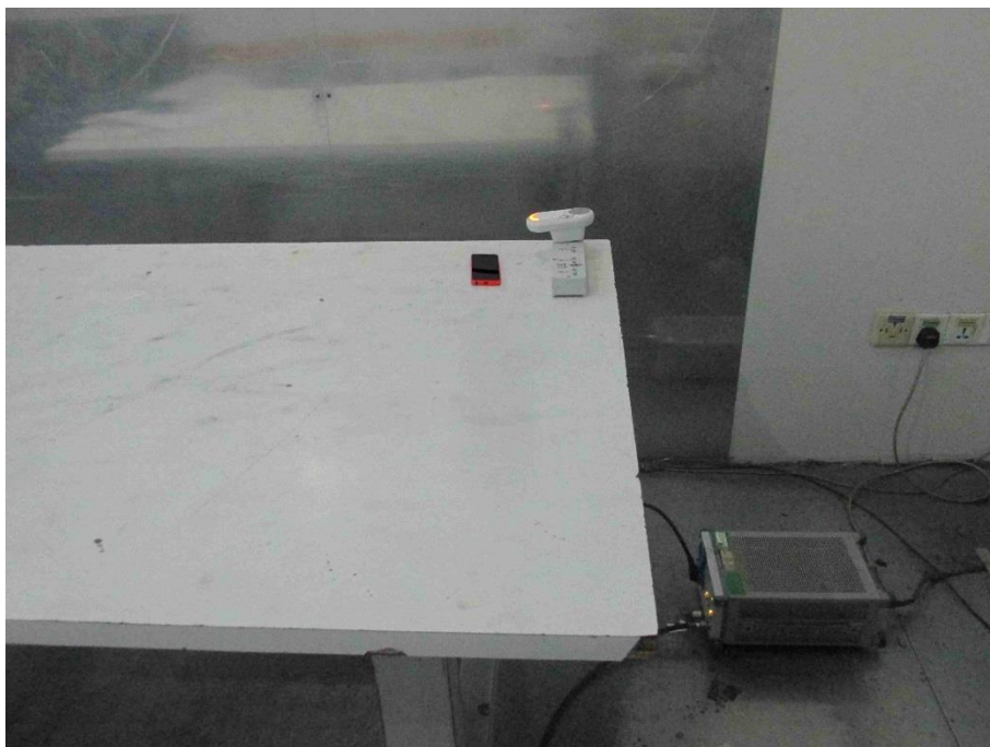
Photograph 4: Set-up for Conducted Emission on AC Mains
