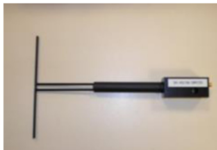
Figure 1 – Satimo COMOSAR Validation Dipole
