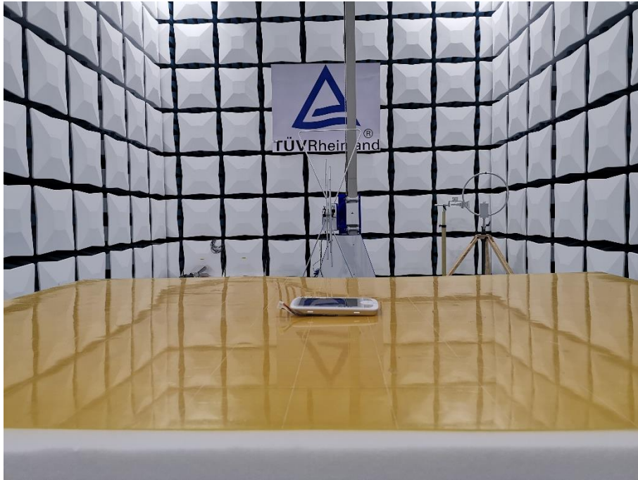
Photograph 1: Set-up for Radiated Spurious Emission, 30MHz - 1GHz
