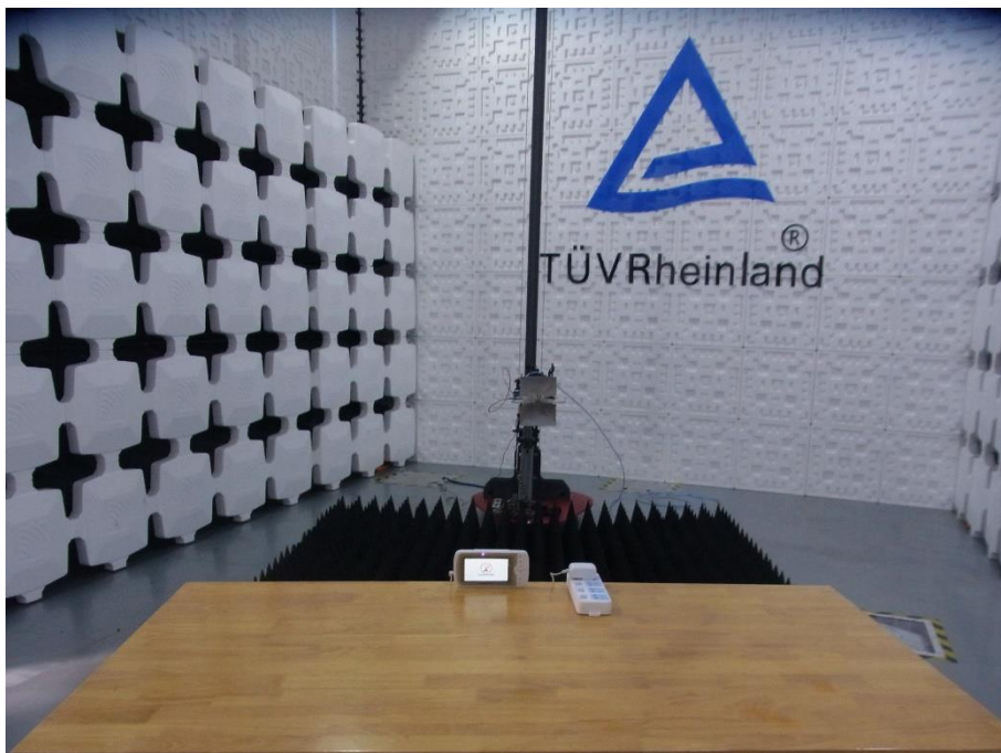
Photograph 5: Set-up for Radiated Emission, Above 1GHz
