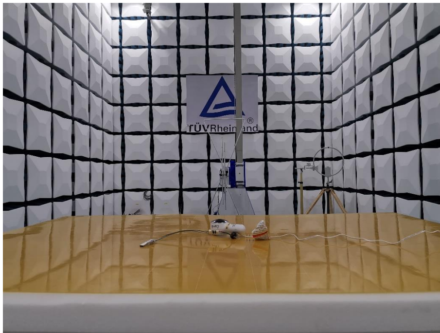
Photograph 1: Set-up for Radiated Spurious Emission, 30MHz - 1GHz
