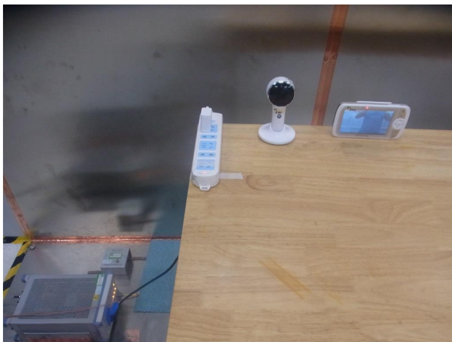
Photograph 3: Set-up for Conducted Emission on AC Mains
