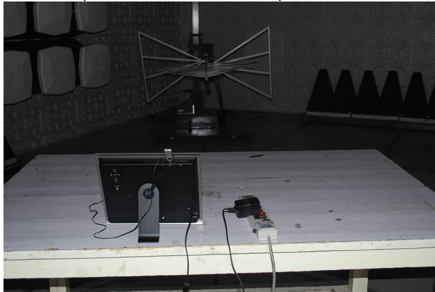
Radiated Spurious Emission Test Setup
