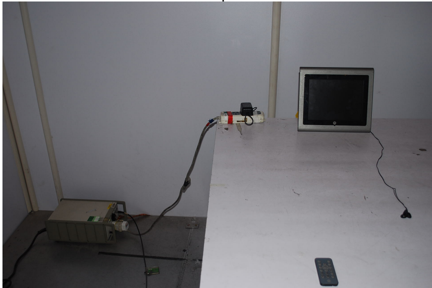
Conducted Emission Test Setup
