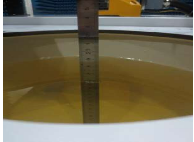
Fig. 9.2 Photo of Liquid Height for Body SAR of Twin Phantom (1900MHz) (depth>15cm)
