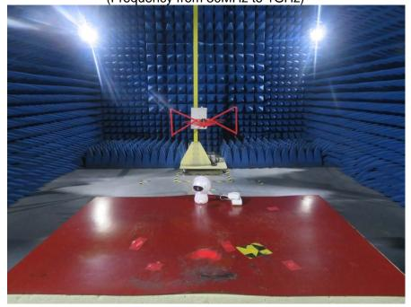
RADIATED EMISSION TEST (Frequency above 1GHz)
