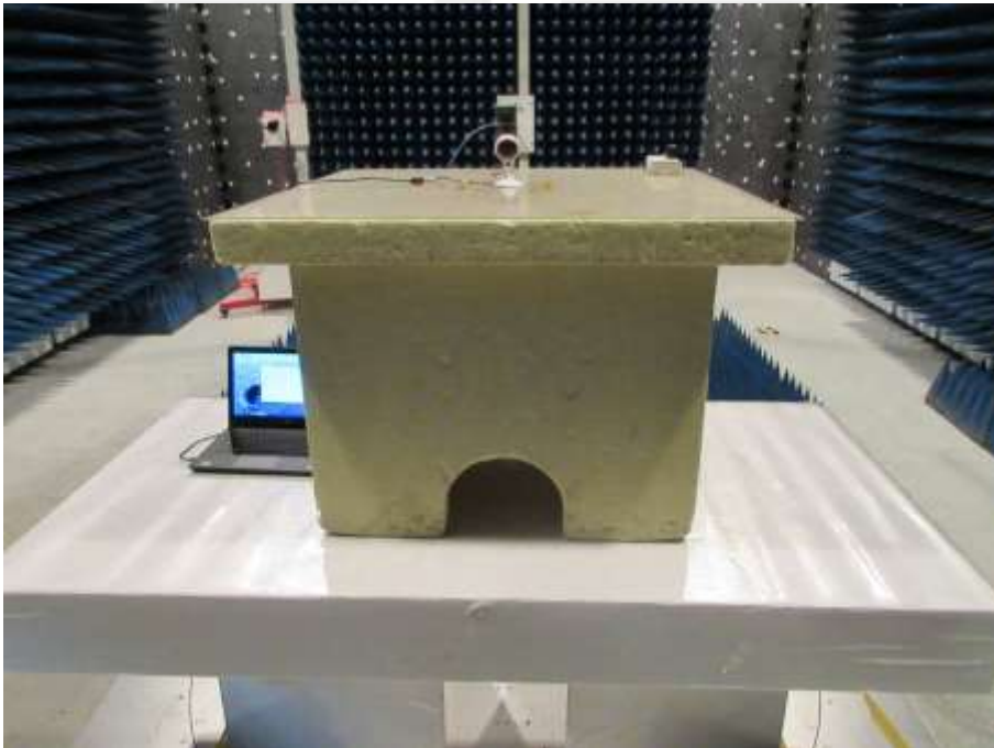
Radiated SPURIOUS EMISSION SET-UP PHOTOS, 1GHz ~ 25GHz
