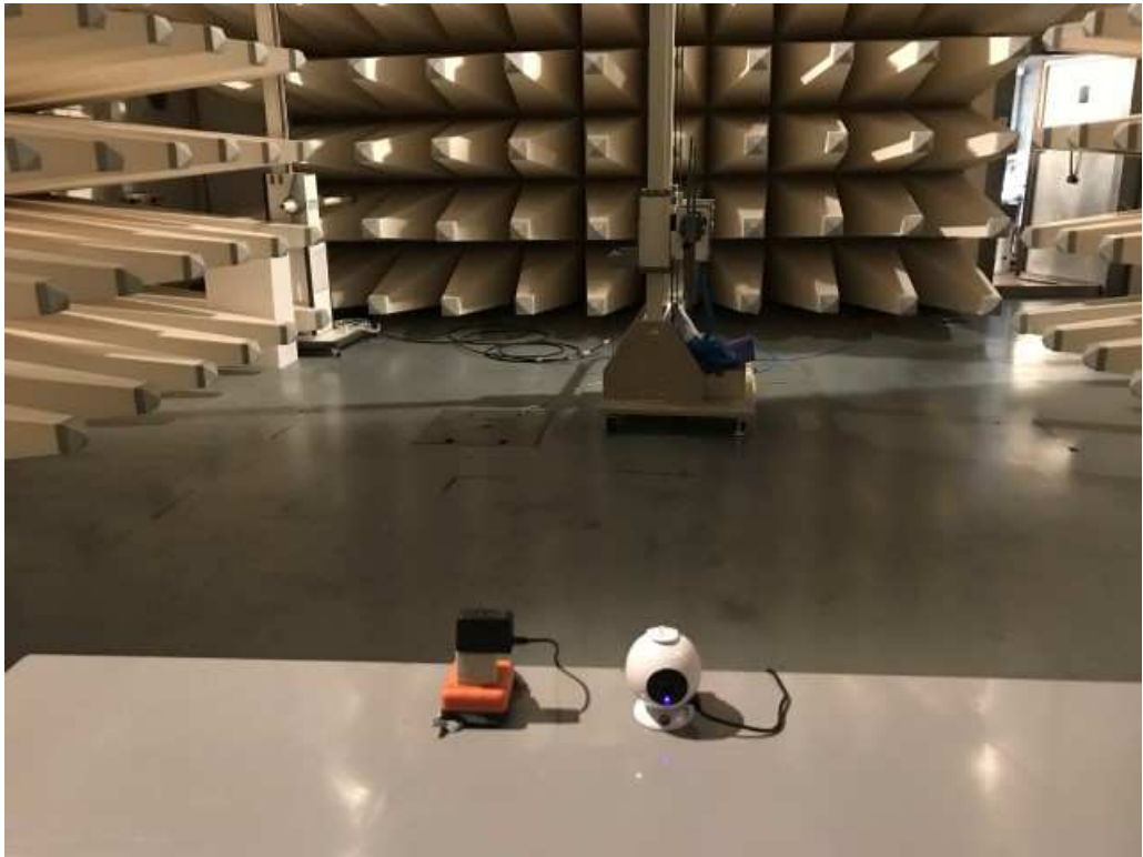
Set-up for Radiated Emission
