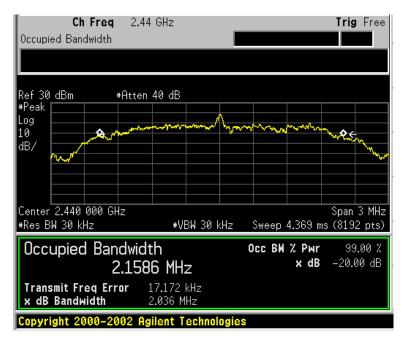
Result data graph shows 20 dB bandwidth, CF = 2440MHz, BW = 2.036MHz
