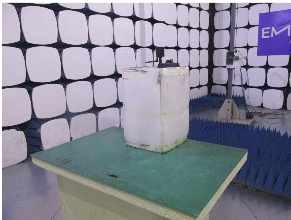
Photograph 2: Set-up for Radiated Spurious Emission, Above 1GHz
