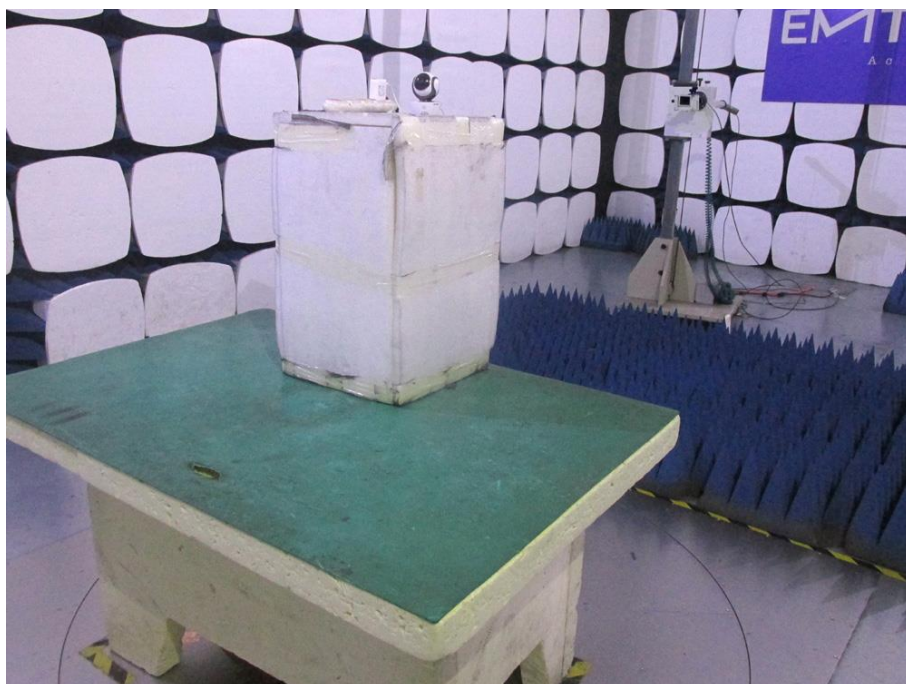
Photograph 4: Set-up for Radiated Spurious Emission, 18GHz - 26.5GHz
