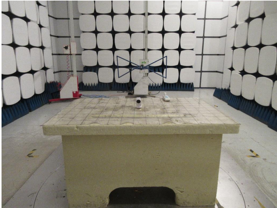
Radiated SPURIOUS EMISSION SET-UP PHOTOS, 30MHz ~ 1GHz
