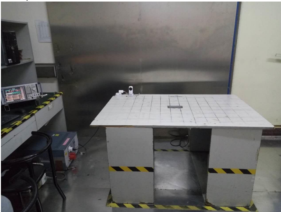
Photograph 4: Set-up for Conducted Emission on AC Mains
