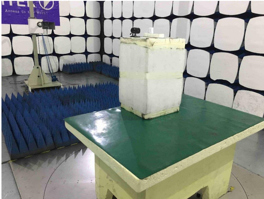
Photograph 3: Set-up for Radiated Spurious Emission, 1GHz - 18GHz
