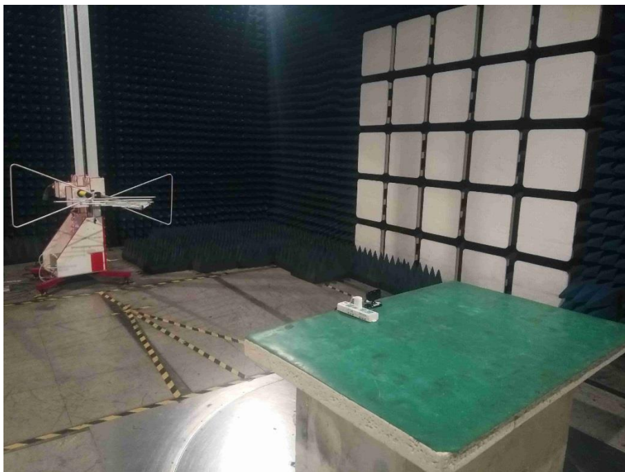
Photograph 2: Set-up for Radiated Spurious Emission, Below 1GHz
