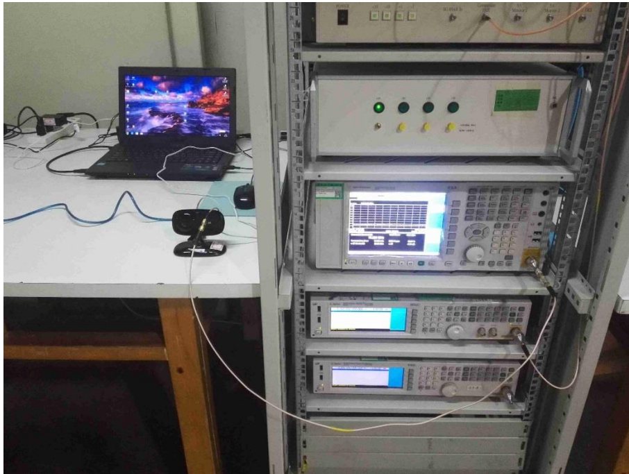
Photograph 1: Set-up for Radio Spectrum Test
