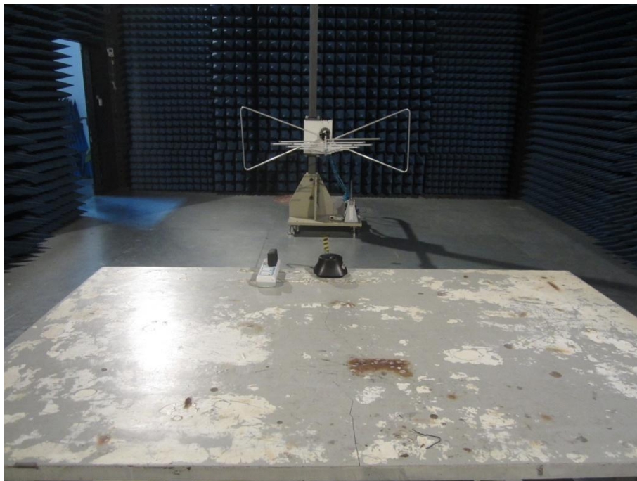
Figure 2 Setup for Radiated Emission(below 1GHz)
