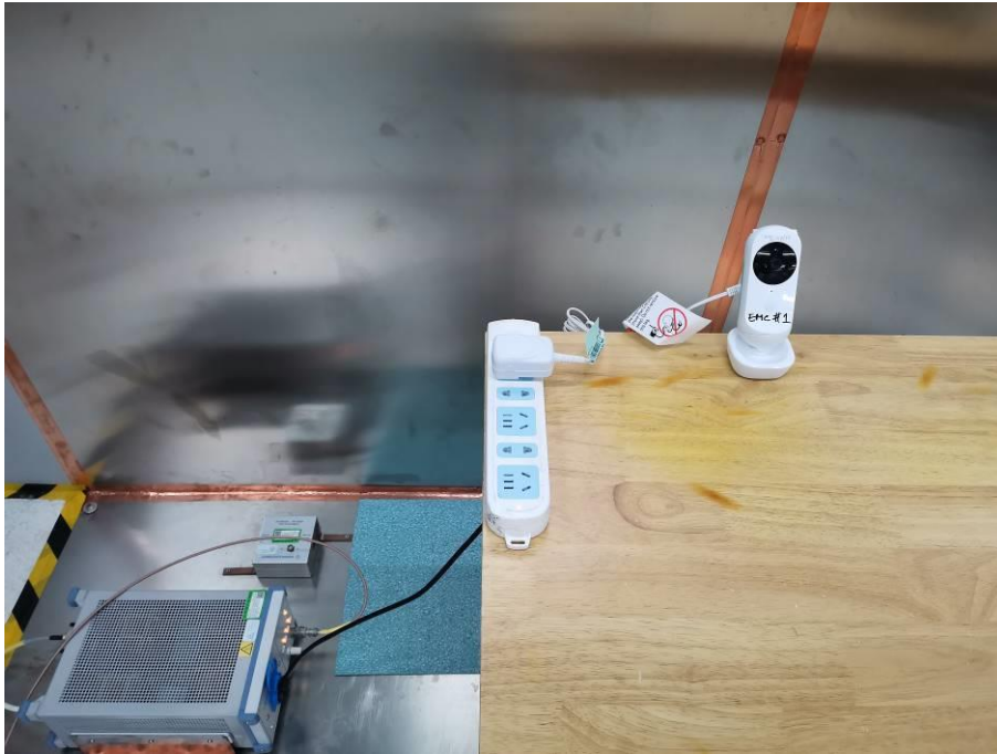
Photograph 4: Set-up for Radiated Emission, Below 1GHz
