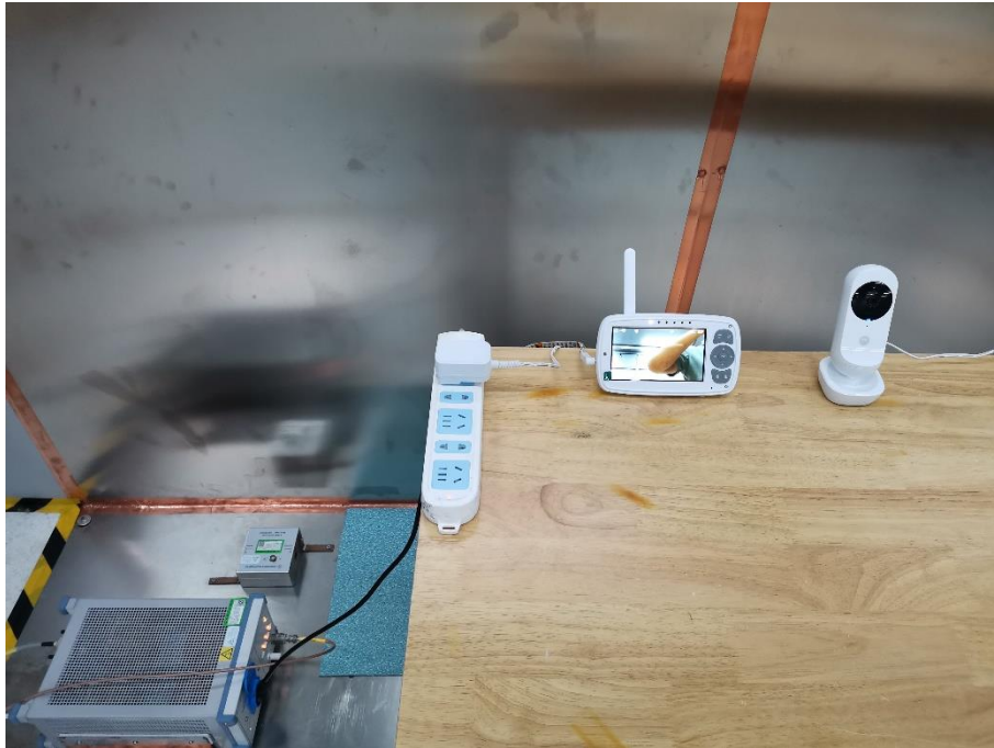
Photograph 3: Set-up for Conducted Emission on AC Mains
