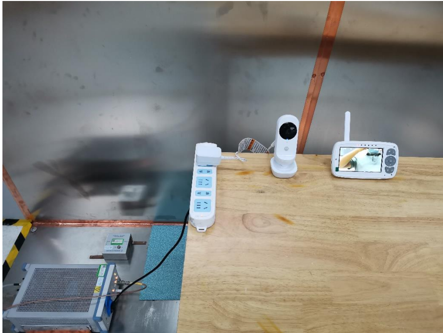
Photograph 3: Set-up for Conducted Emission on AC Mains
