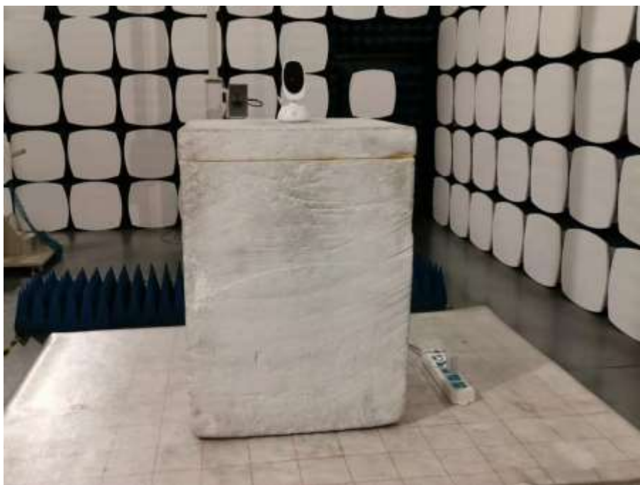
Radiated SPURIOUS EMISSION SET-UP PHOTOS, 1GHz ~ 25GHz
