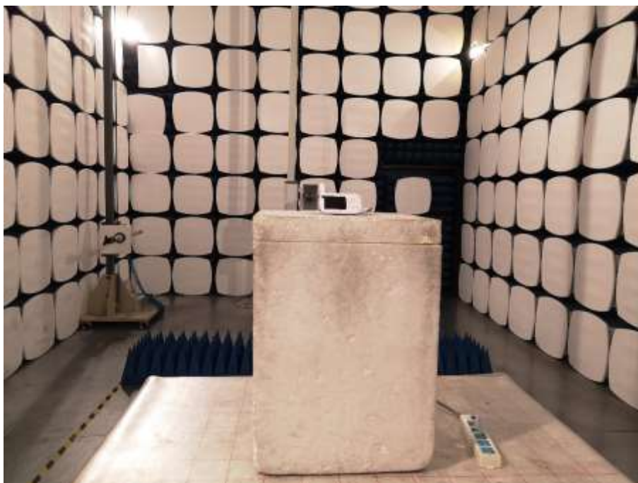
Radiated SPURIOUS EMISSION SET-UP PHOTOS, 1GHz ~ 25GHz
