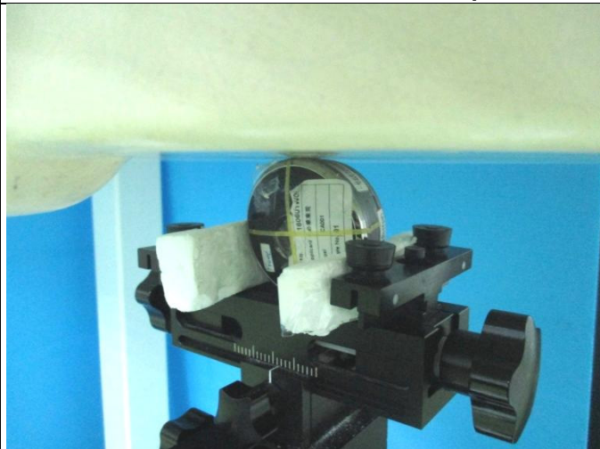
Right Side of EUT with 0 cm Gap
