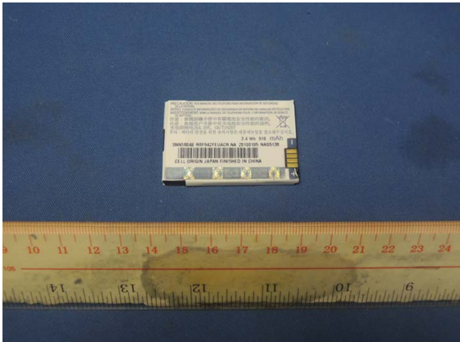
Figure 4 – 3.7VDC 910mAh Lithium-ion rechargeable battery back view
