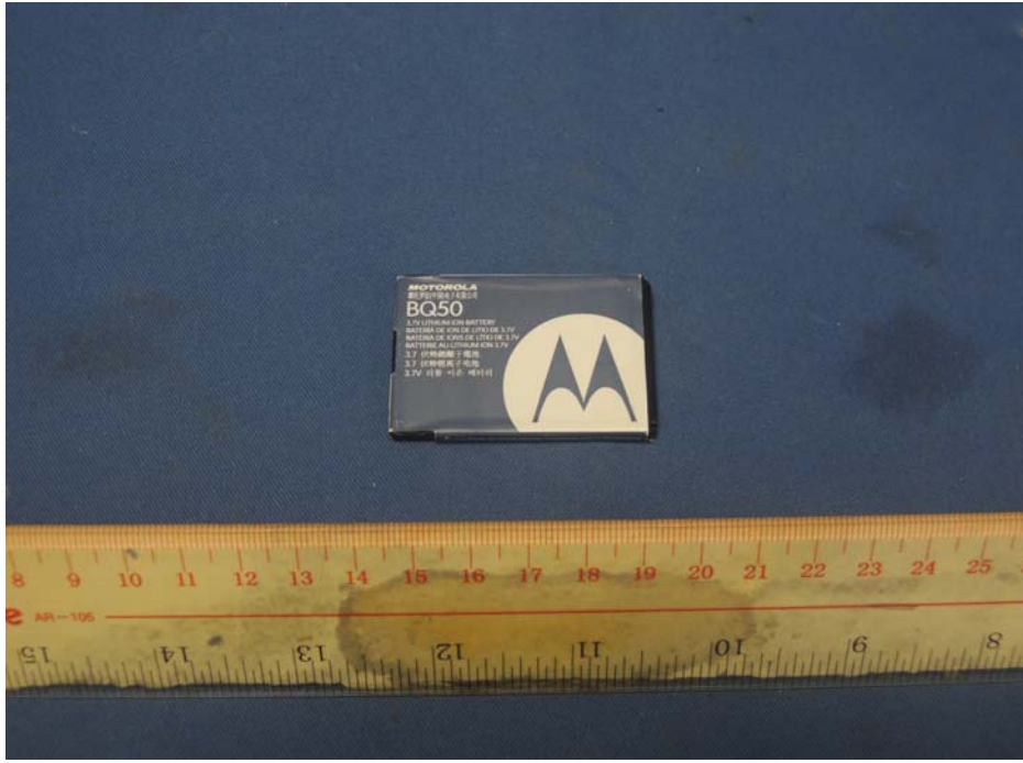
Figure 3 – 3.7VDC 910mAh Lithium-ion rechargeable battery front view
