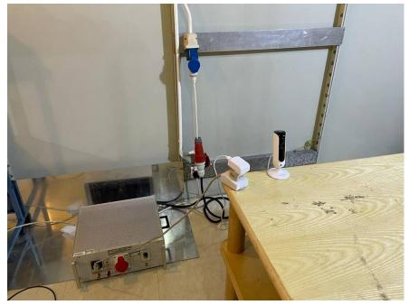
Radiated Emissions (30MHz-1GHz) Test Setup
