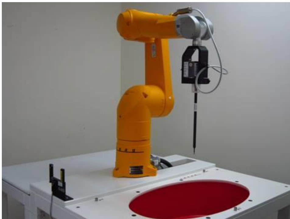
Fig.1 Photograph of the SAR measurement system
