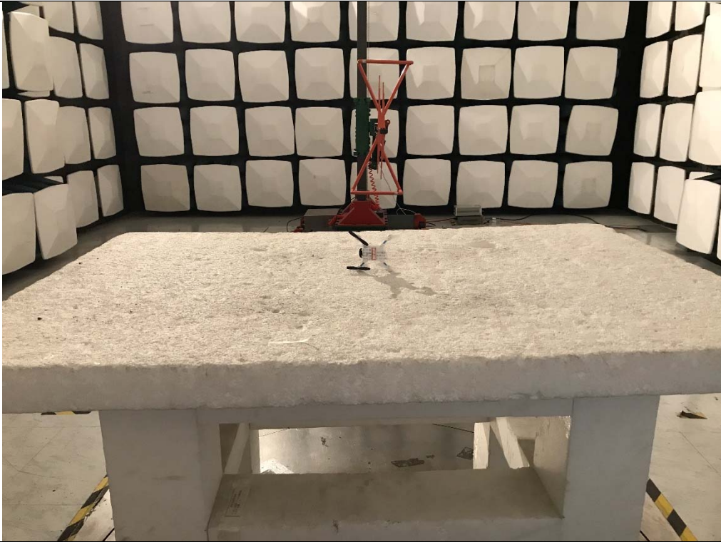
Radiated emission Test Setup-1 (30 MHz~1 GHz)
