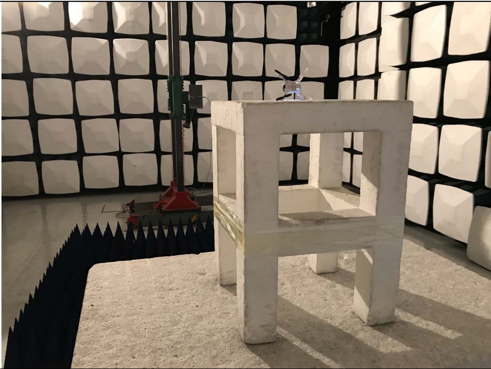
Radiated emission Test Setup-2 (Above 1 GHz)
