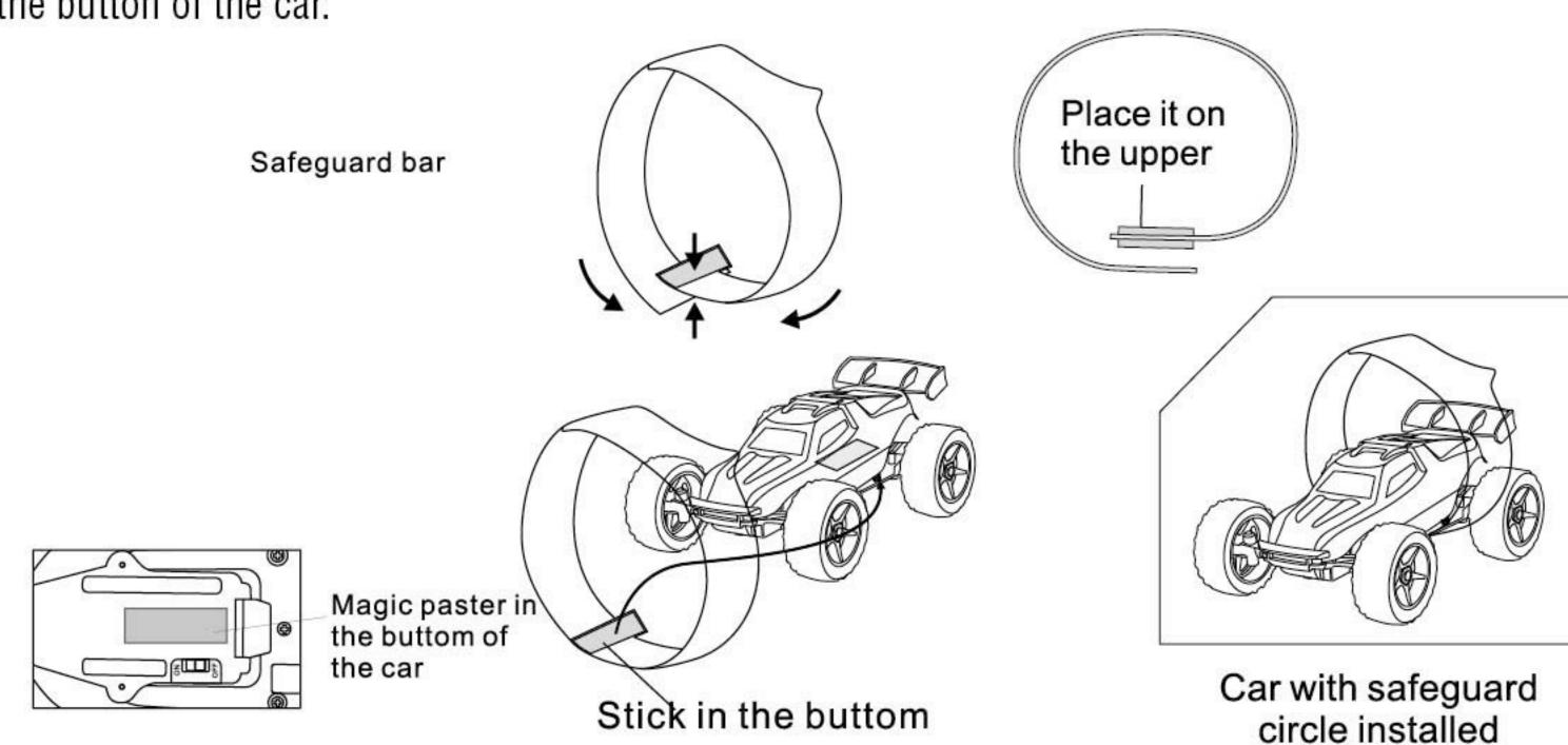
The car with protect ring can rolling-over and keep going when it turned over.
