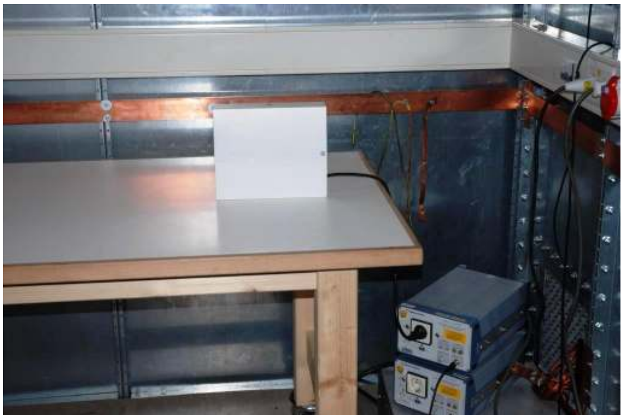
Fig.3 Conducted emission setup
