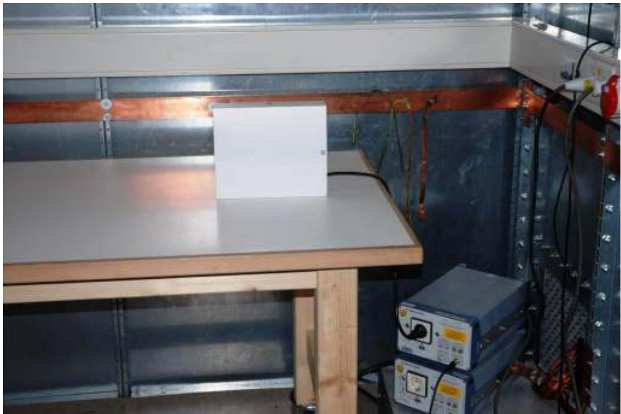
Fig.3 Conducted emission setup
