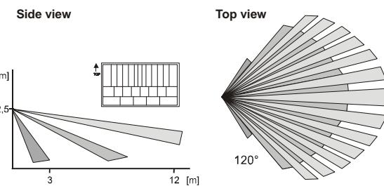
The characteristics can be changed by using optional lenses:
