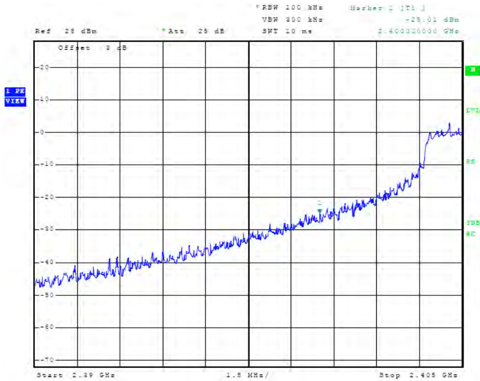
Figure 97 Plot of Low Band Edge Compliance at Antenna Port (chain2, 2.4MHz Operation)
