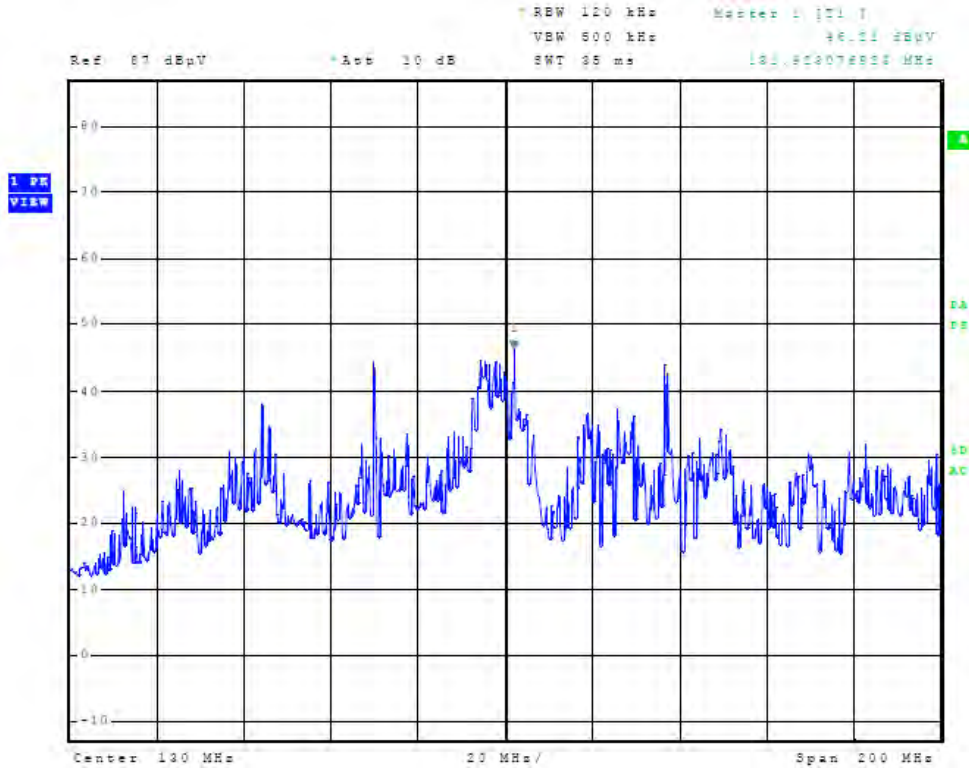
Figure 3 General Radiated Emissions taken at 1 meter in screen room
