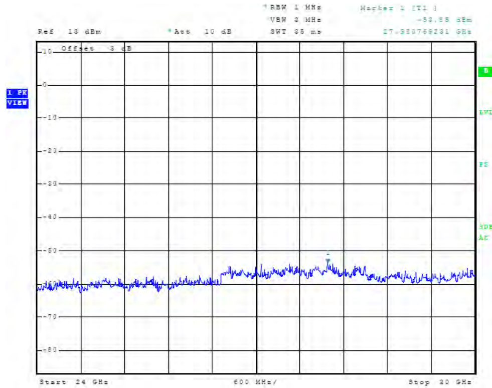
Figure 67 Plot of Antenna Port Conducted Emissions (5 GHz, chain 1, operation)
