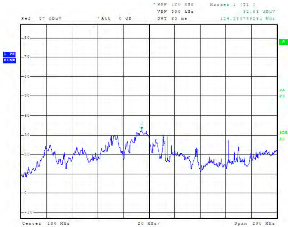
Figure 137 Plot of Receiver Radiated Spurious Emissions taken at 1 meter
