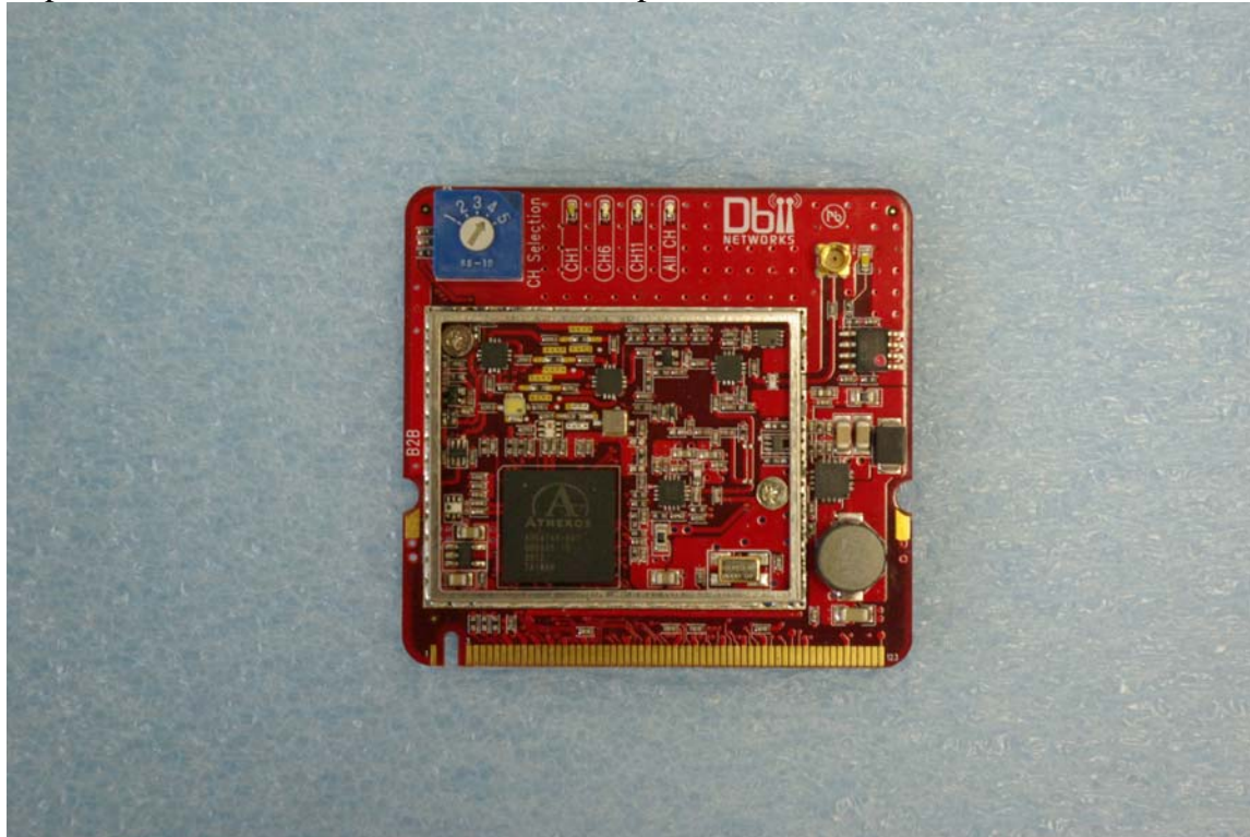
Internal photographs of equipment under test Top of Transmitter module without shield in place
