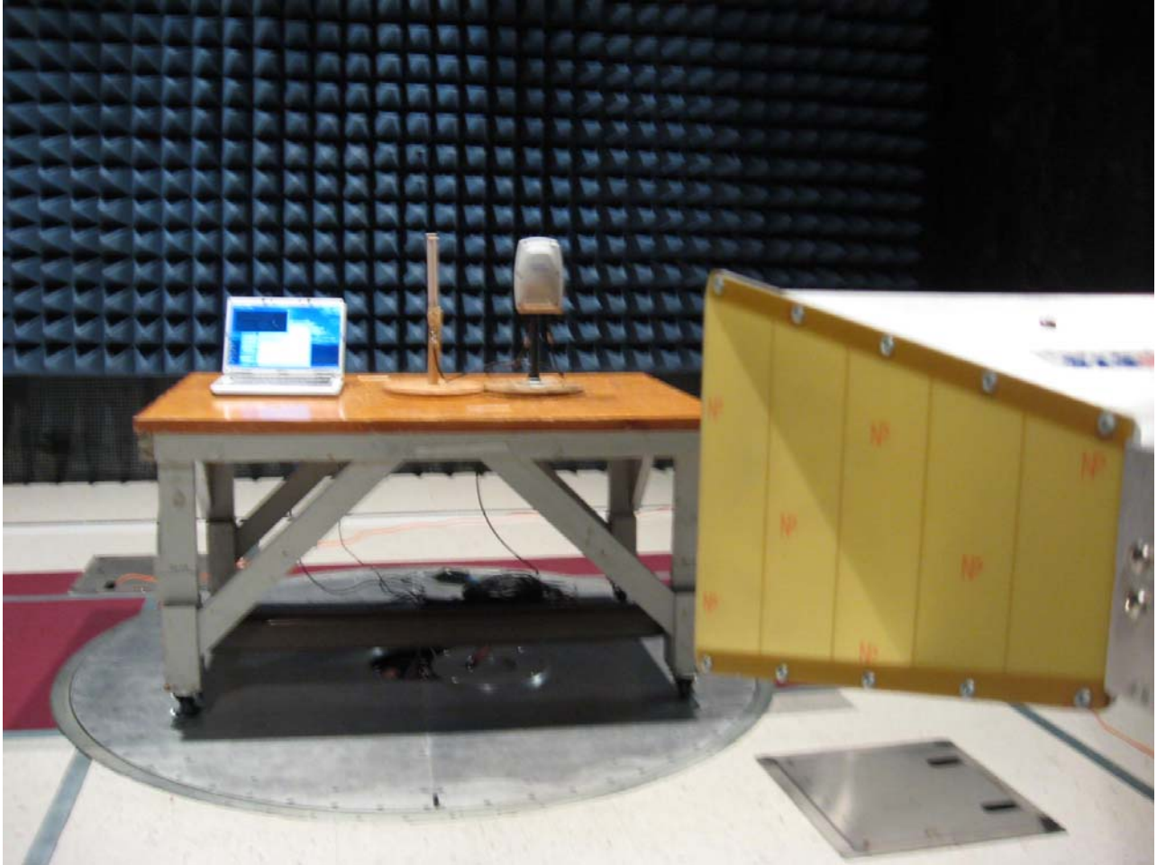
Photograph 1. Test Equipment and setup for various Radiated Measurements
