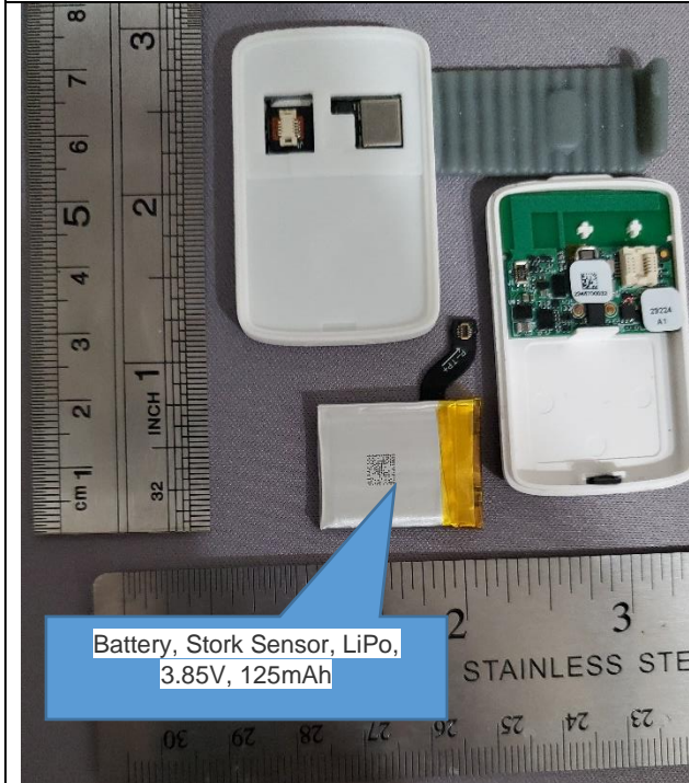
Photo 2: Internal view of Baby sensor with the battery removed
