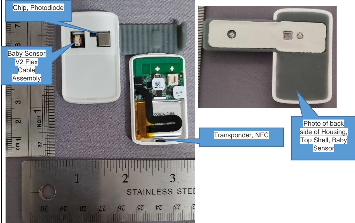
Photo 2: Internal view of Baby sensor with the battery removed
