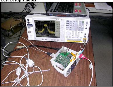
**Test Conditions:** The EUT is on the table and all the probes and cables are connected to the unit. Measurements are made by direct connect with the Serial cable connected to the laptop computer, which is used to change the TX characteristics.
