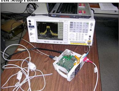
**Test Conditions:** The EUT is on the table and all the probes and cables are connected to the unit. Measurements are made by direct connect with the Serial cable connected to the laptop computer, which is used to change the TX characteristics. The 3 channels in the 5.2 GHz range were tested against the 50mW limit. The 3 channels in the 5.8 GHz range were tested against the 1 W limit.
