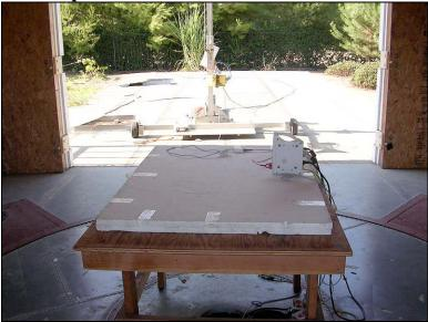
**Test Conditions:** The EUT is on the table and all the probes and cables are connected to the unit. Measurements are made by direct connect with the Serial cable connected to the laptop computer, which is used to change the TX characteristics.
