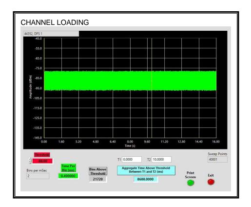
The level of traffic loading on the channel by the EUT is 86.88%.
