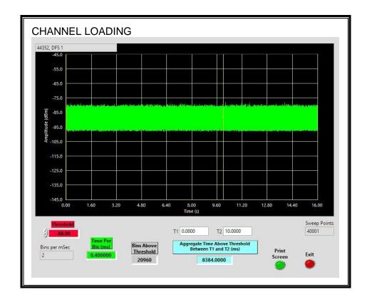
The level of traffic loading on the channel by the EUT is 83.84%.
