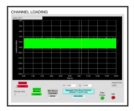
The level of traffic loading on the channel by the EUT is 80.488%.
