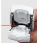
Once the finger is correctly positioned, gently close the MightySat by releasing the pressure on the back of the device. 5.
