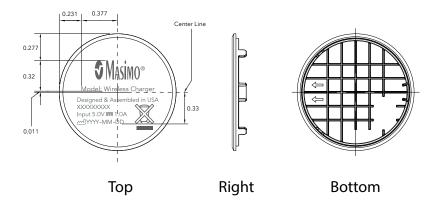
Inspection Dimensions dimensions in inches tolerance +/- 0.015"
