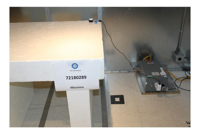
AC Conducted Emissions Test Setup
