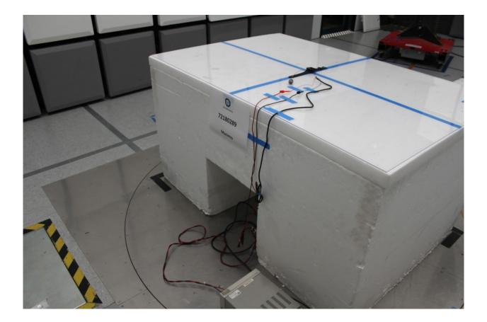
Cabinet Spurious Emissions Radiated Test Setup
