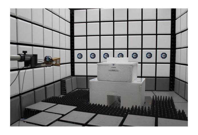
Radiated Emissions Test Setup (18GHz TO 40GHz)
