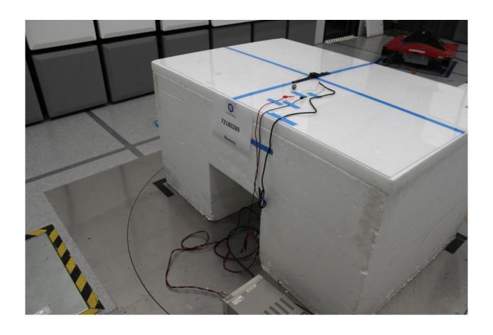
**Cabinet Spurious Emissions Radiated Test Setup**
