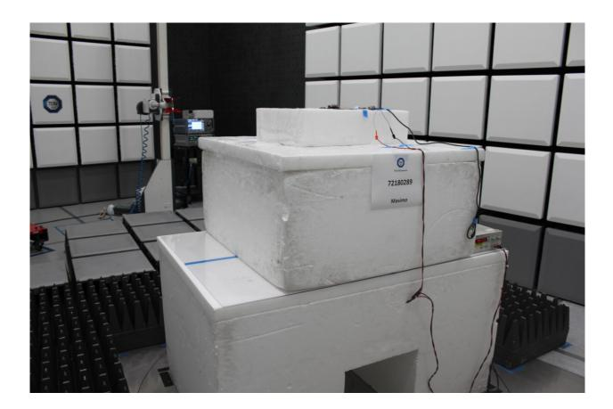
Radiated Emissions Test Setup (1GHz to 18GHz)
