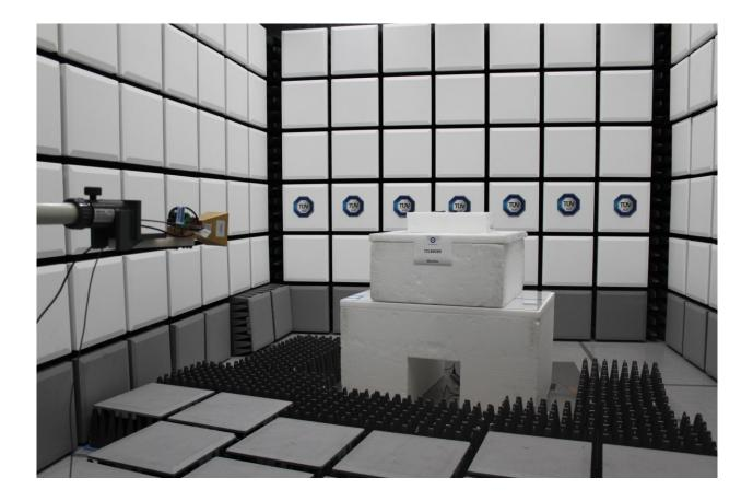
Radiated Emissions Test Setup (18GHz TO 40GHz)
