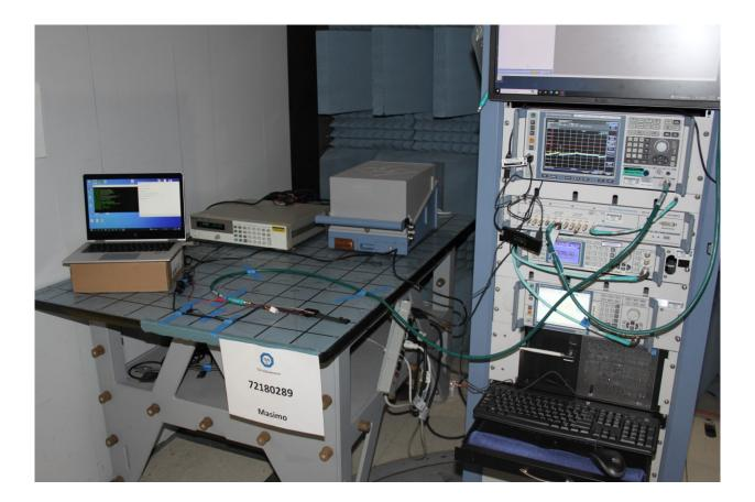
Antenna Port Conducted Test Setup
