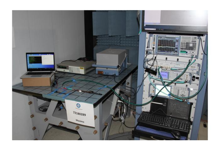
**Antenna Port Conducted Test Setup**
