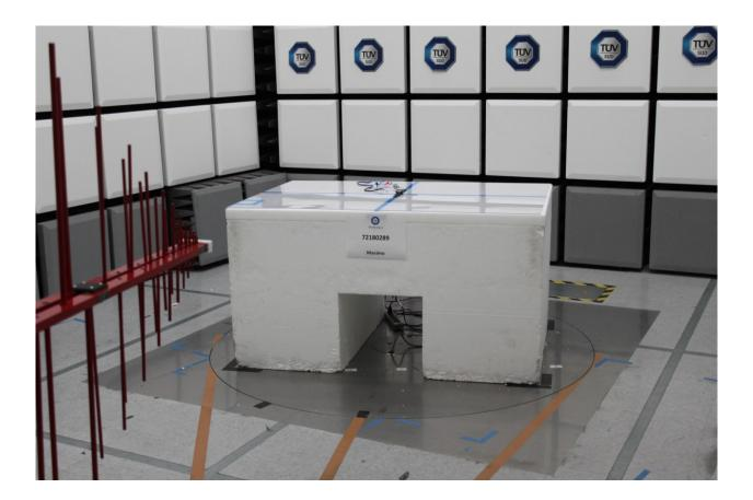
Radiated Emissions Test Setup (30MHz to 1GHz)
