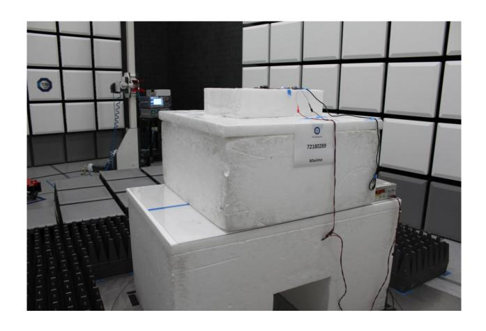
Radiated Emissions Test Setup (1GHz to 18GHz)
