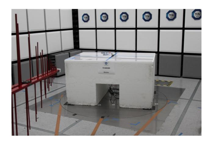
Radiated Emissions Test Setup (30MHz to 1GHz)
