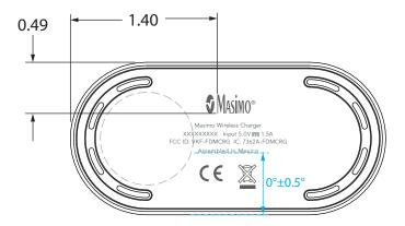
Inspection Dimensions dimensions in inches tolerance +/- 0.030"
