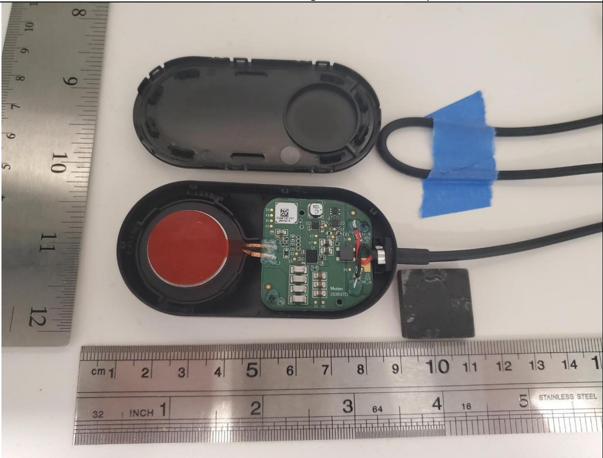
Closer view of Internal view of Masimo Wireless Charger with the cover open
