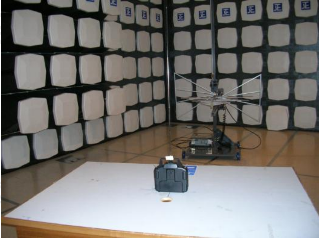
Measurement of Radiated Emission Test Set Up
