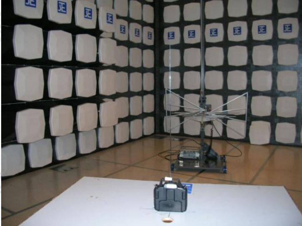
Measurement of Radiated Emission Test Set Up
