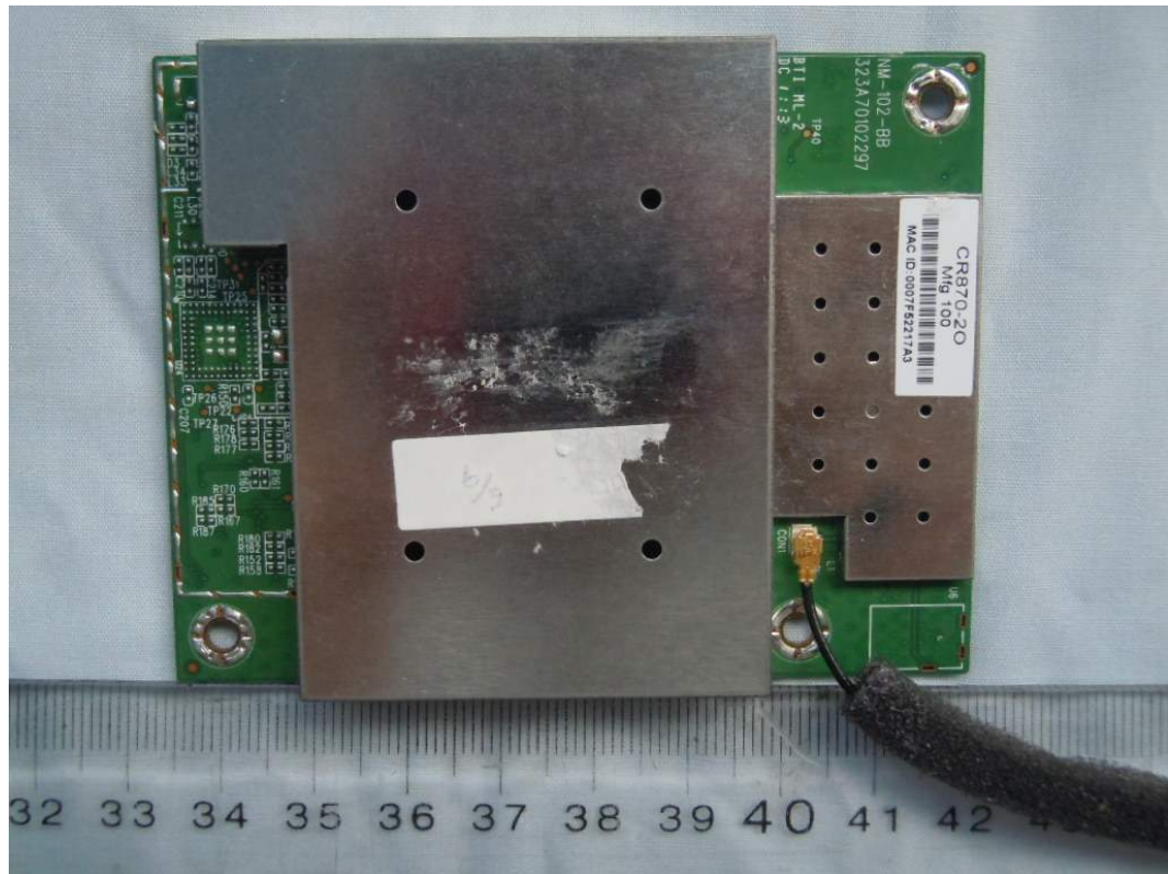
FIGURE 6 WIRELESS AIRPLAY SPEAKER (M/N: MA5000) RF BOARD (COMPONENT SIDE)
