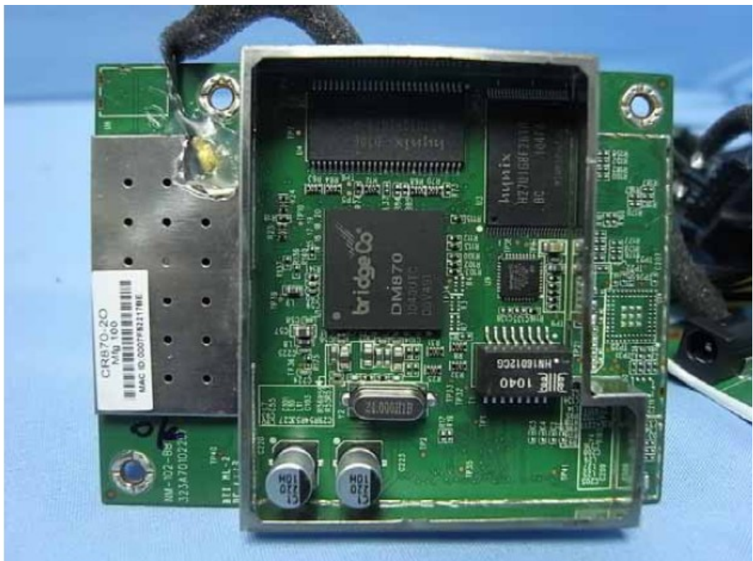
FIGURE 7 WIRELESS AIRPLAY SPEAKER (M/N: MA5000) RF BOARD (SHIELDED COVER REMOVED #1)
