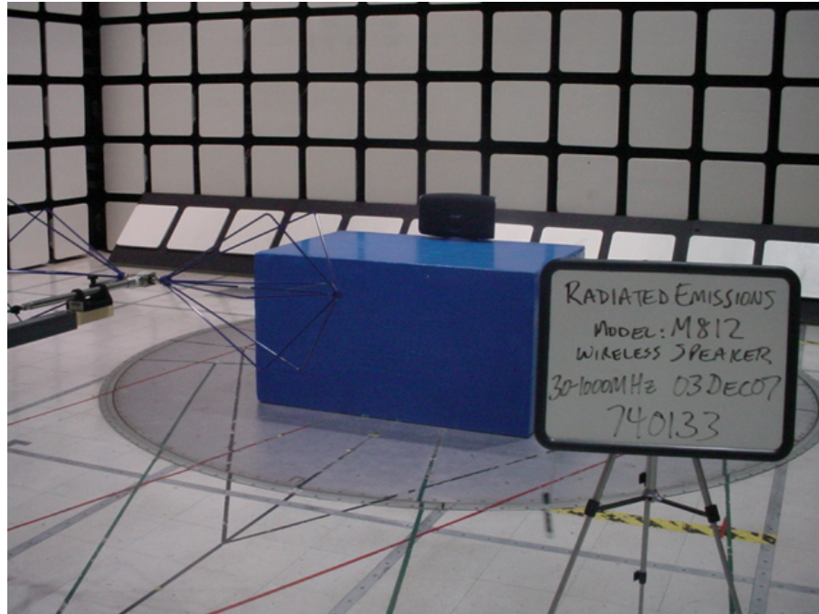
Figure 25 Test setup for Radiated Emissions (30-1000MHz) – Wireless Speaker
