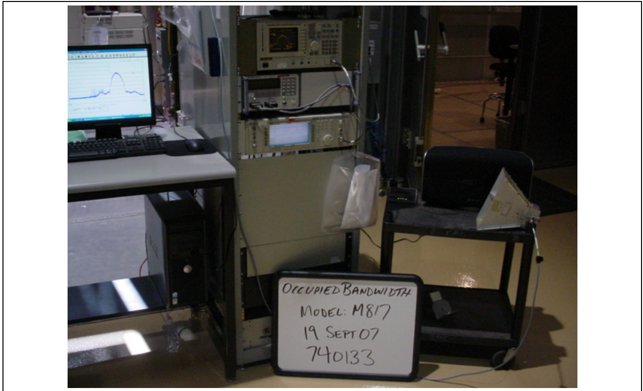
Figure 8 Test Setup for Occupied Bandwidth
