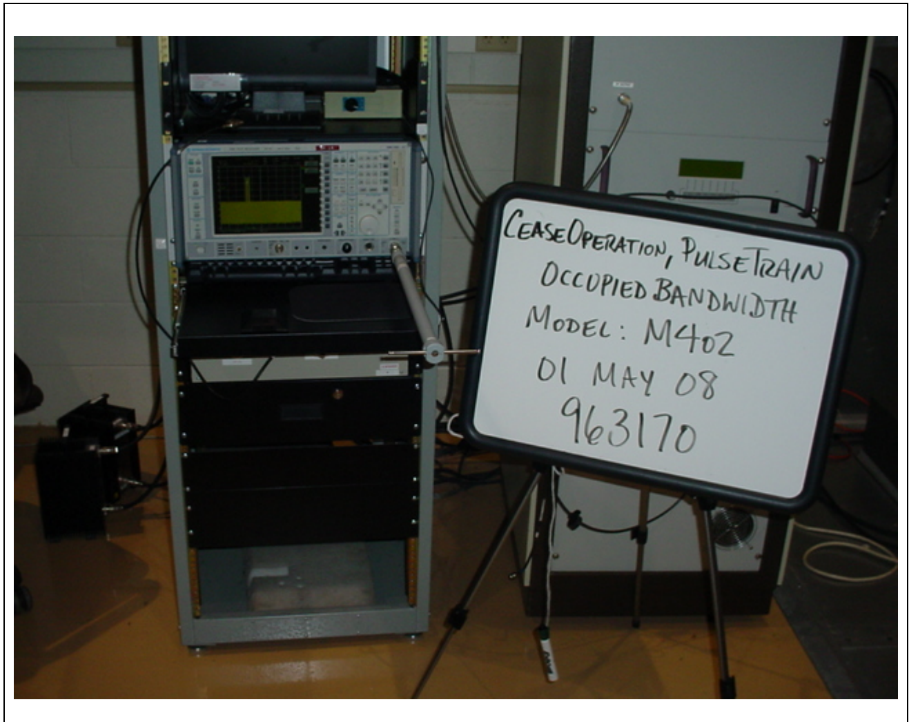
Figure 3 Test Setup for Occupied Bandwidth
